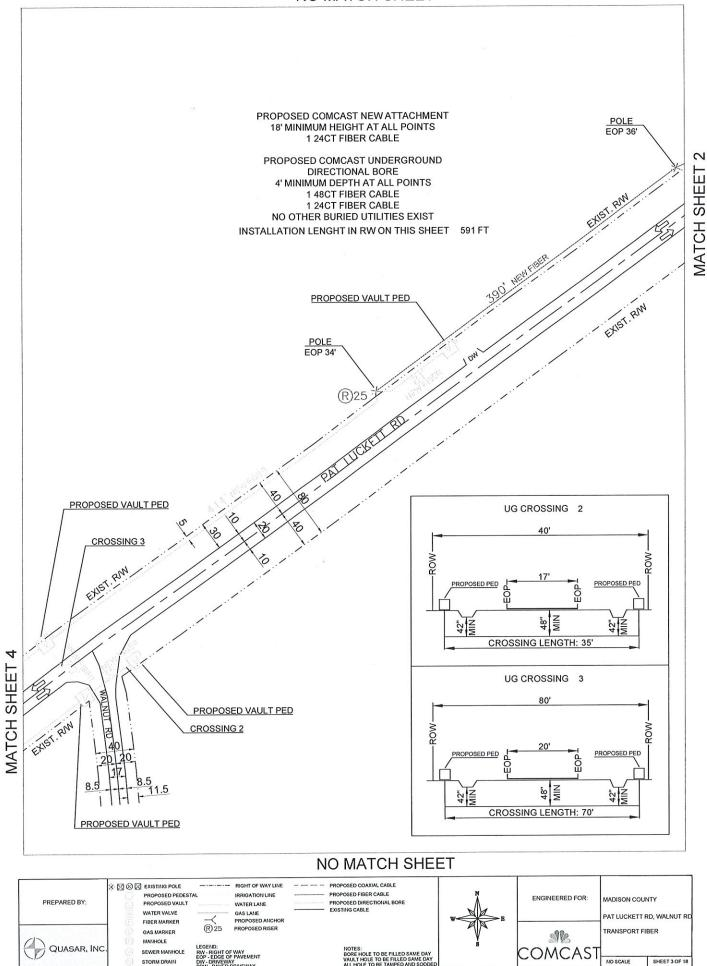
PROPOSED COMCAST UNDERGROUND DIRECTIONAL BORE 4' MINIMUM DEPTH AT ALL POINTS 1 48CT FIBER CABLE NO OTHER BURIED UTILITIES EXIST
